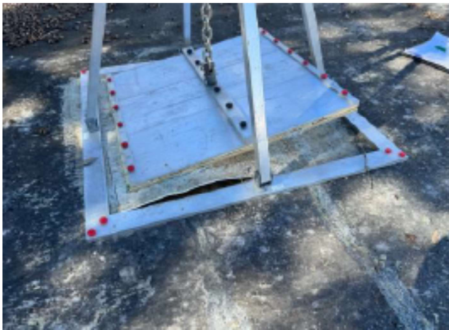
Bonded uplift test at point of failure.
